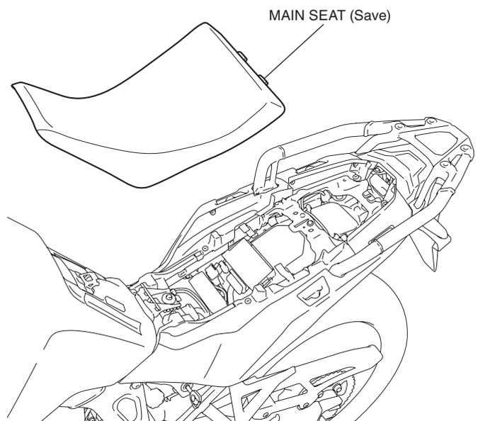
3. Install the main low seat in the reverse order of removal.
